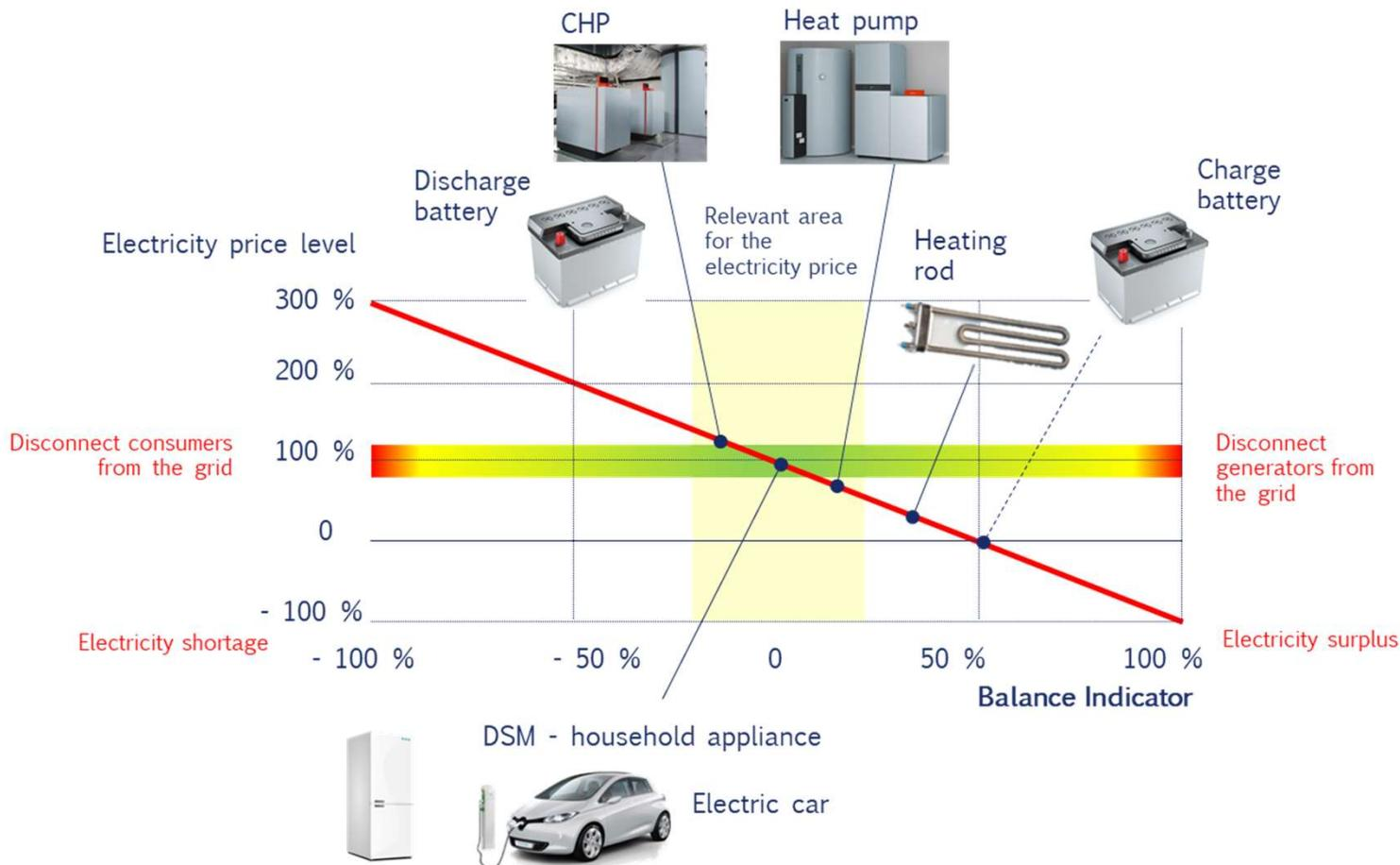
Easy Smart Grid technology allows to integrate and reward flexible energy consumption/generation into the electric grid ensuring system stability and data security. Individual flexible resources receive direct incentives to change their consumption patterns, by a balance indicator derived from physical network variables such as frequency or the terminal voltage. The system reacts immediately to information on variations in the grid.
