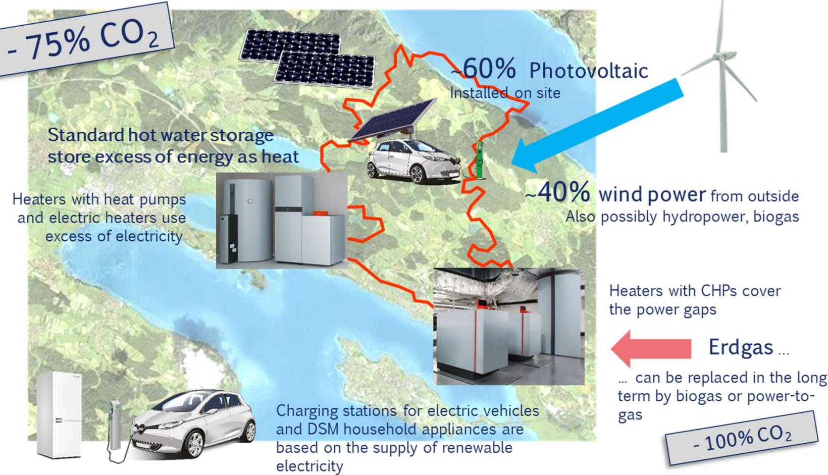
As a result of the heating/cooling and electricity sector coupling, around 80% of the solar and wind energy can be coupled into the local power grid. With a mix of 60% locally generated PV and 40% external wind power, the power grid needs only little expansion.
